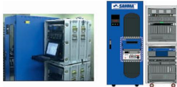
Fig 5. Robot and control system developed by Media Matters and commercialised under the name of Samma System.
